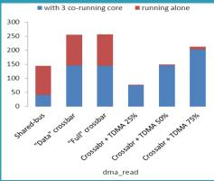
Interference measurement on a SoC demonstration platform
